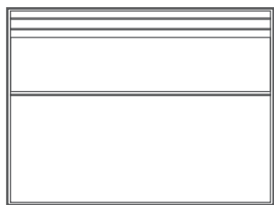
top: accessory rail middle: tackable fabric bottom: laminate panel
